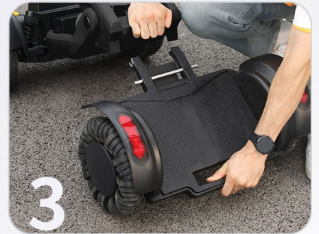
3 Press down on the chassis quick release area and pull out the pedal assembly
